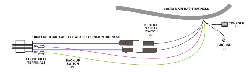
1. On page number 3 of the main dash harness kit, P/N 510065, locate Items number 19 and 20. Items 19 are the back up lamp switch wiring, and items 20 are the neutral safety switch wiring.
