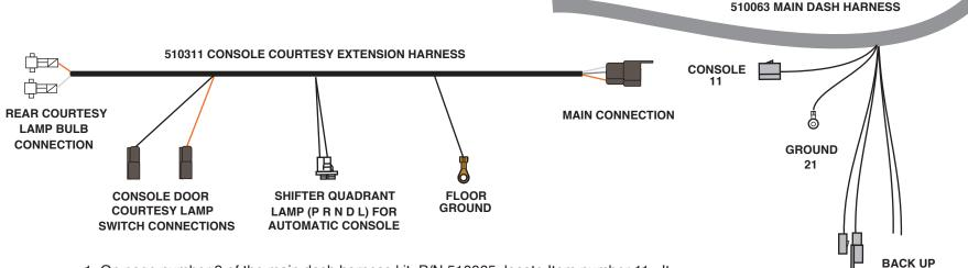
1. On page number 3 of the main dash harness kit, P/N 510065, locate Item number 11. It is a 3 way connector containing orange, white, and gray wires. This is your main console connection.
